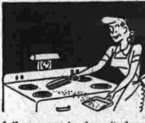
ood or liquid spills on open coil type of surface unit, shut off current and remove residue with soft brush. Flat-bottomed utensile are suggested for best efficiency.
